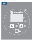
01 = Switching Status Indicator 99 = Right button 20 = Enter Button A0 = Detachable li 22 = UP Button 60 = Display
